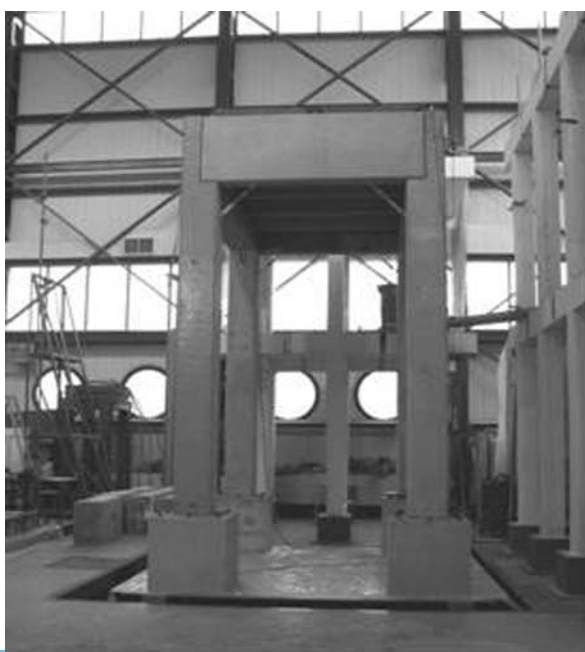
Fig. 10.16 Reduced-scale mock up of a precast building designed and built for shaking table testing at LNEC for the “Growth-PRECAST EC8” research project
