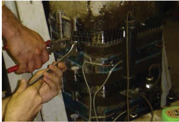
Fig. 6.5 Method of pre-stressing (See also Plate 7 in Color Plate Section on page 459)
