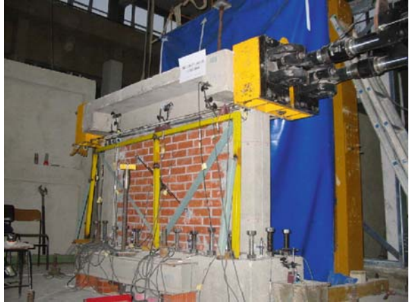
Fig. 19.12 Testing set-up and integrated wall (See also Plate 31 in Color Plate Section on page 472)
