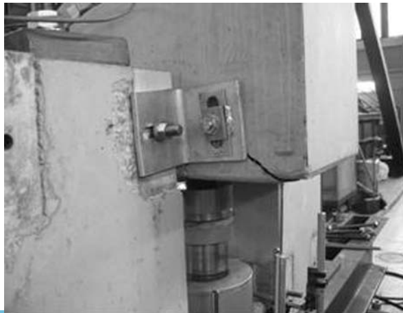
Fig. 10.24 Failure mechanism of the specimen (spalling of cover concrete)
