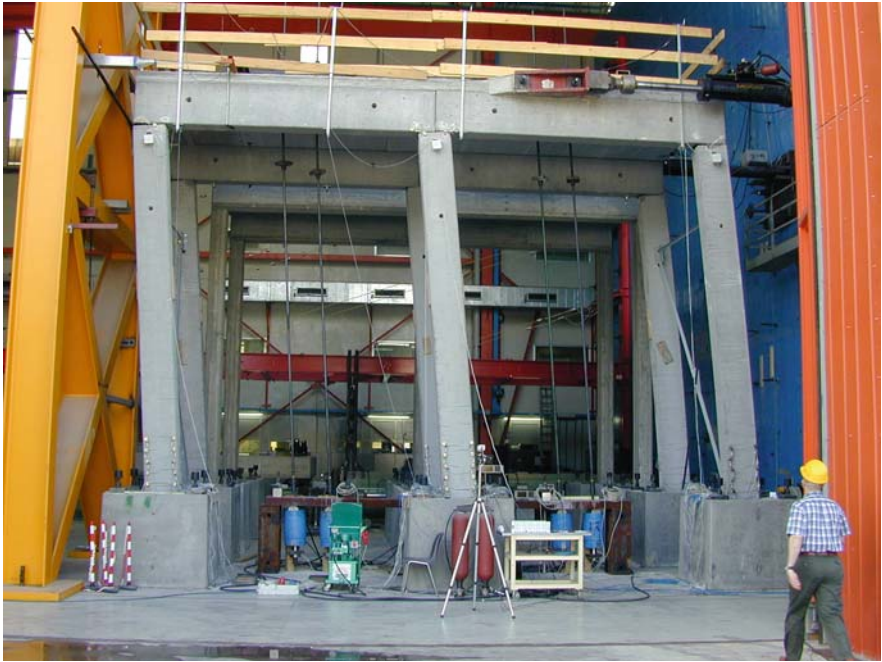
Fig. 10.12 Precast mock up for pseudodynamic testing designed and built for the “Ecoleader” research project
