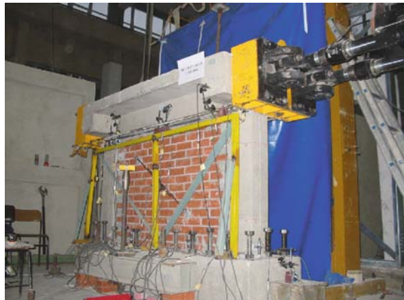
Plate 31 Testing set-up and integrated wall (see also Fig. 19.12 on page 398)
