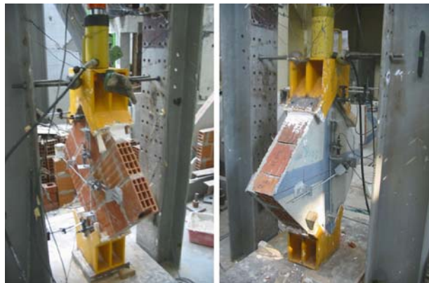
Plate 29 Pure shear tests of brittle walls (see also Fig. 19.7 on page 393)
